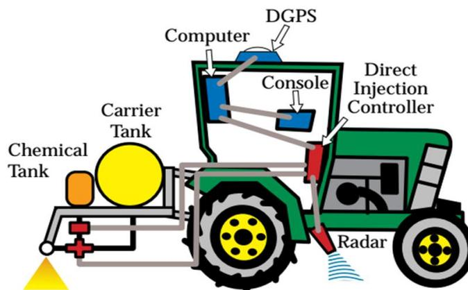
**Figure-2.** Representation of the components of the variable rate technologies for chemical application.
