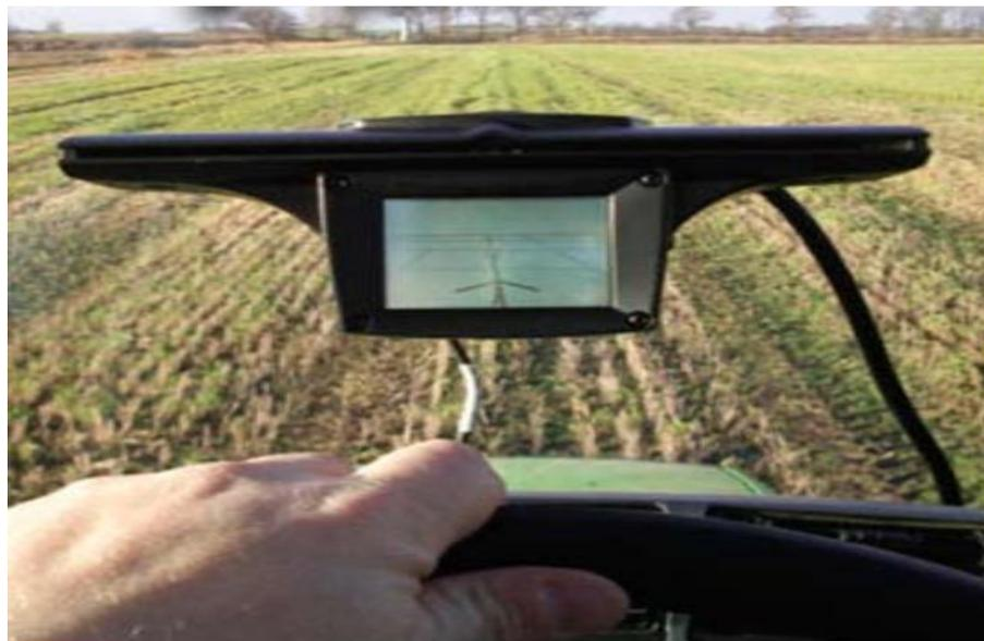
**Figure-1.** An example of a light bar guidance system.
